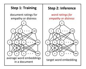
Figure 1: Schematic illustration of the MLFFN: **Step 1** Train a model to predict a document rating from the embedding of the document text; **Step 2** "Invert" the trained model to compute a word rating for each word embedding.
