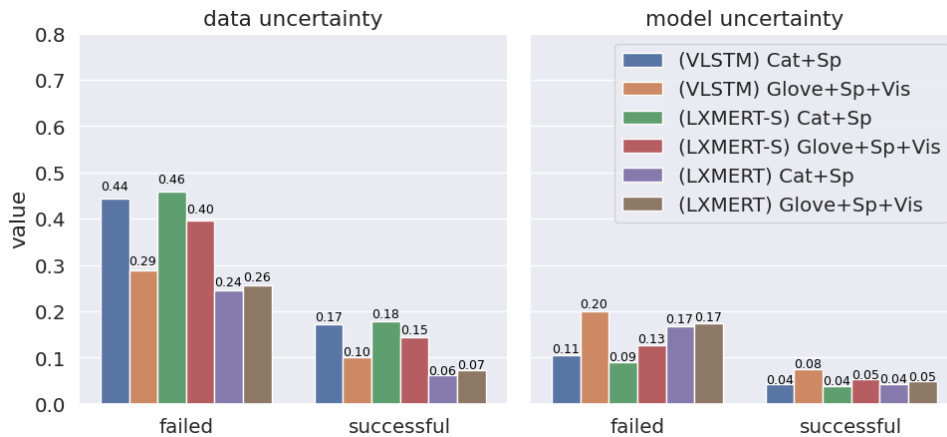
Figure 3: Total, data, and model uncertainty for different ensembles considering games with 5 candidate objects. Improved candidate representations decreases data uncertainty for V-LSTM, but not for LXMERT or LXMERT-scratch.
