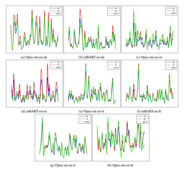
Figure 3: Comparison of time-duration across source, target and prediction for all of the aforementioned models as well as languages (de, fr, ru, it, hi) using Amazon Polly text-to-speech API. Here y-axis represents the duration of speech and *Blue*, *Red*, and *Green* lines show the time duration taken by the model for uttering the source text, target text, and generated isometric translated text.
