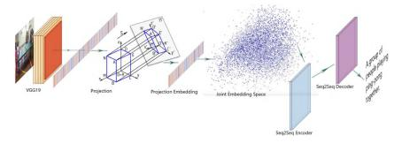
Figure 4: Architecture of Image captioning using IMAGINATOR. We use VGG19 for embedding and then we use IMAGINATOR to project into the joint embedding space. We pick K nearest objects/words and pass to seq2seq model to generate caption.
