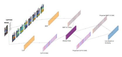
Figure 7:  $BERT_{IMAGINATOR}$  - Training approach for Image Retrieval. Training happens in batches and cosine similarity between corresponding image-sentence pair is maximised while for other pairs it is minimized.
