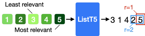
Figure 2: Two variants of LISTT5, ( r=1 ) and ( r=2 ). The underlying model is identical and only the inference method varies. ( r=1 ) keeps only the top 1 relevant index from the output, and ( r=2 ) keeps top 2 relevant indices.
