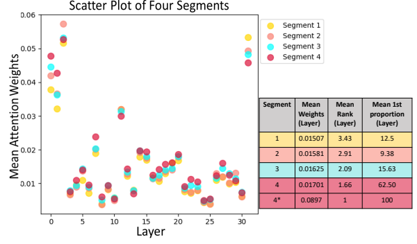
Figure 3: Scatter Plot of the average attention weights over 256 sentences at every layer. We divide the tokens into four segments based on token entropy, with segment 1 having the lowest entropy and segment 4 the highest (To mitigate the attention sink effect, we omitted the first token in Segment 1 to 4 and Segment 4* stands for segment 4 with the first token). Mean Weights stands for the average attention weights across all layers. Mean Rank denotes the average ranking of each segment at every layer. Mean 1st proportion denotes the proportion of times each segment ranked first across all layers. The figure indicates that as token entropy increases, so does the attention that the LLM allocates to that token.
