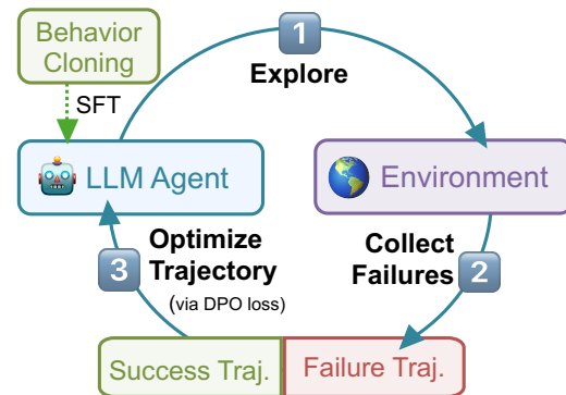
Figure 1: Exploration-based Trajectory Optimization (ETO) allows an LLM agent to iteratively collect failure trajectories and update its policy by learning from contrastive failure-success trajectory pairs.
