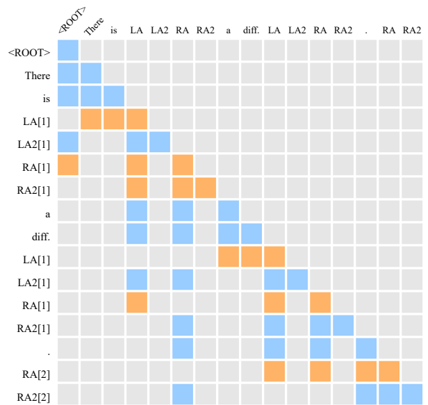
(b) Attention mask. Tokens are simplified for a tight view. We use orange to represent COMPOSE and blue to represent STACK . The number in [] is the ARC number of LEFTARC/RIGHTARC.
