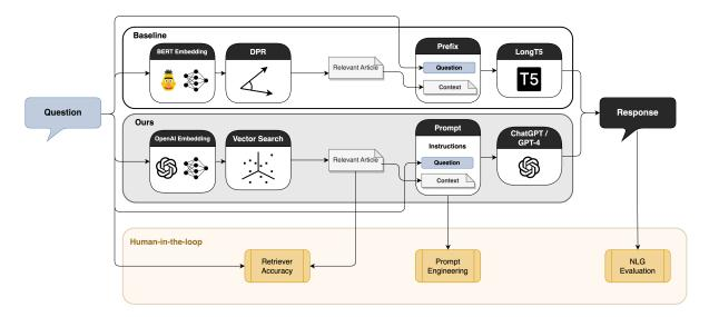
Figure 2: Block diagram of the methodology introduced in our paper, illustrating baseline and Open AI models, highlighting the role of the human-in-the-loop during development
