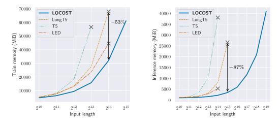
Figure 4: Memory consumption during a typical training (forward + backward) (**left**) and inference iteration (only forward) (**right**). Batch size = 1. Ending cross means out-of-memory or architectural limitations after this point.
