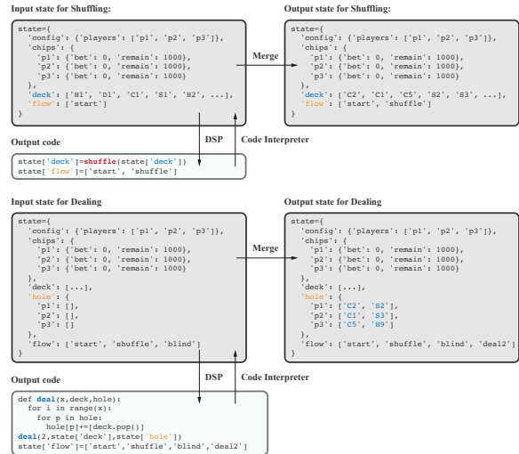
Figure 3: DSP. In the shuffling case, the IDGE calls “shuffle”, which is a predefined core function. In the dealing case, it defines a new “deal” function to deal a number of cards to each player one by one. We use a code interpreter to merge the input state and the output code to obtain the next state.
