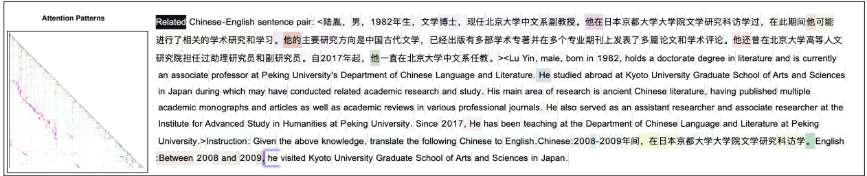
Figure 2: Average attention scores of the final layer of the Qwen-14B-Chat model. The darker the color, the higher the attention score assigned to that token. It is noteworthy that the model attends to “他” (meaning “he” in English) from the examples we extract when generating “he”. Our examples successfully help the model in translating the zero pronoun “他” (meaning “he” in English).
