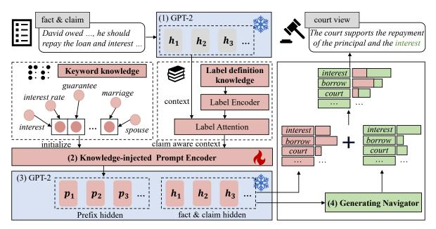
Figure 2: The architecture of KIG. (1) is the frozen pretrained GPT-2, utilized for obtaining input context. (2) is the knowledge-injected prompt encoder, which incorporates claim knowledge to obtain claim-aware context. (3) is the same frozen GPT-2, which is used for calculating the activation of output from the knowledge-injected context. (4) is the generating navigator, guiding the model's inference process.
