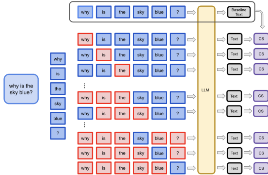
Figure 1: Flowchart of the TokenSHAP algorithm illustrating the process of Shapley value estimation for token importance in large language models by accepting parts of the text to the players and a cosine similarity measure to the base prompt as a gain.
