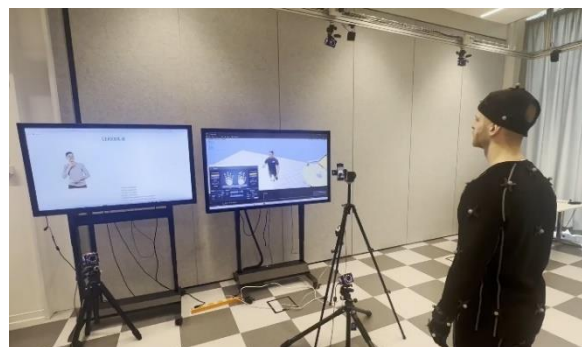
Figure 4: The set-up for recording motion capture data for lexical signs.
