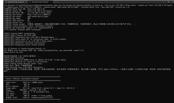
Figure 3: Live OpenGlass run in an Anaconda prompt showing end-to-end instrumentation (audio receive, ASR, Wi-Fi capture, image packing, VLM TTFT/total, and TTS). These auditable logs support both reproducible evaluation and failure analysis.
