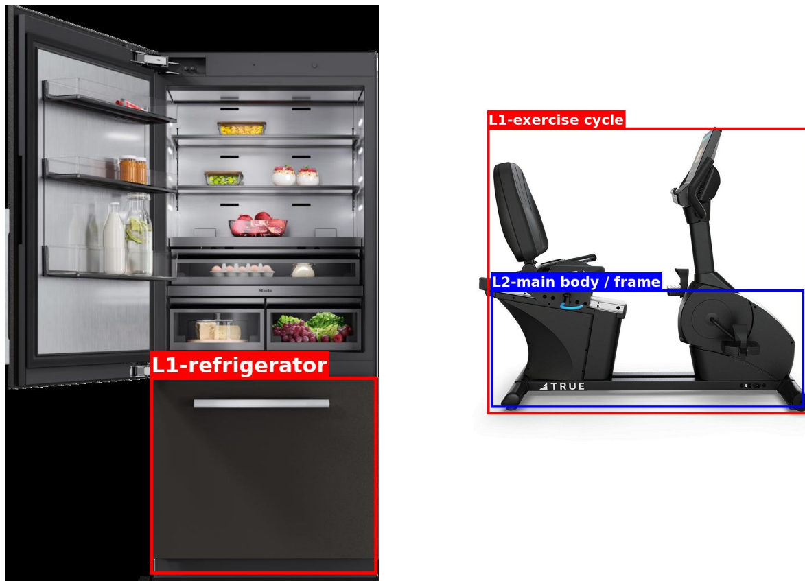
Figure 8: Failure Case 1: Cascading errors from parent misclassification. When the model misclassifies an L1/L2 to a small bounding box, child components like door (left) and seat (right) are omitted due to hierarchical validation.
