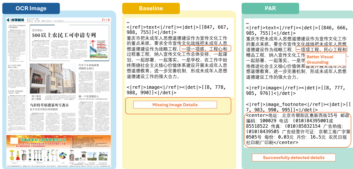
Figure 12: Qualitative comparison on OmniDocBench (Case 2). This example highlights the model's ability to handle complex layouts. The baseline model fails to ground the visual content effectively, missing entire blocks of text and image details. With PAR, the model exhibits stronger visual grounding, successfully detecting and transcribing the fine-grained footnotes and layout structures that were previously ignored.
