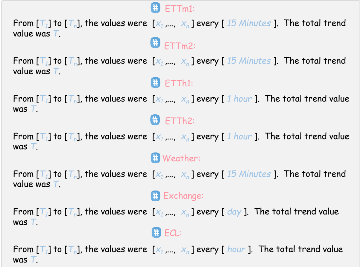
Figure 6: Hint templates for specific datasets are used to transcribe multivariate time series segments into natural language descriptions. Each template jointly encodes the time interval, numerical sequence, sampling frequency, and trend statistics to establish a unified representation between structured time series data and language model input.
