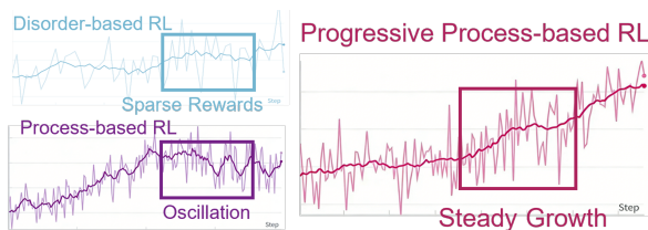
Figure 9: Comparison of three reward strategies during reinforcement learning. The progressive process-based reward yields a smoother and more stable training trajectory compared to disorder-based and fixed process-based rewards.
