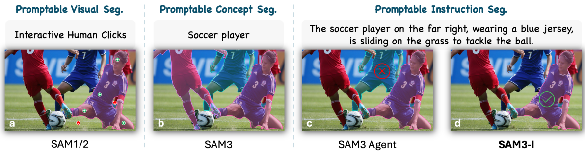
Figure 1: Evolution of promptable segmentation in the SAM family. (a) Promptable Visual Segmentation (PVS) in SAM1/2 relies on interactive visual prompts, with each prompt segmenting a single object. (b) Promptable Concept Segmentation (PCS) in SAM3 supports short NPs as prompts (e.g., “soccer player”) to segment all instances of a given concept. (c) To handle complex natural-language instructions, SAM3 relies on external multi-modal agents to convert instructions into short NPs, which remain overly coarse to capture fine-grained conditions (red icon). (d) Promptable Instruction Segmentation (PIS) in SAM3-I directly interprets complex instructions and grounds the intended target instance (green icon). SAM3-I introduces a unified framework, as the first of its kind in the SAM family, that integrates concept-level understanding and instruction-level reasoning.
