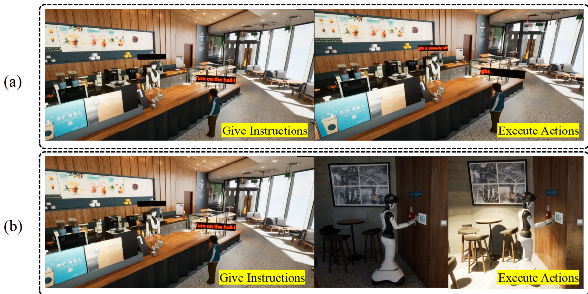
Figure 4: An use example of the robot executing tasks following the customer’s instruction. In (a), the RAG LLM planner is used, and the robot incorrectly informed the guest, "The hall light is already off." which was a misinterpretation of the intended instruction. In (b), the CDRs LLM planner is used and the robot turns on the hall light correctly.
