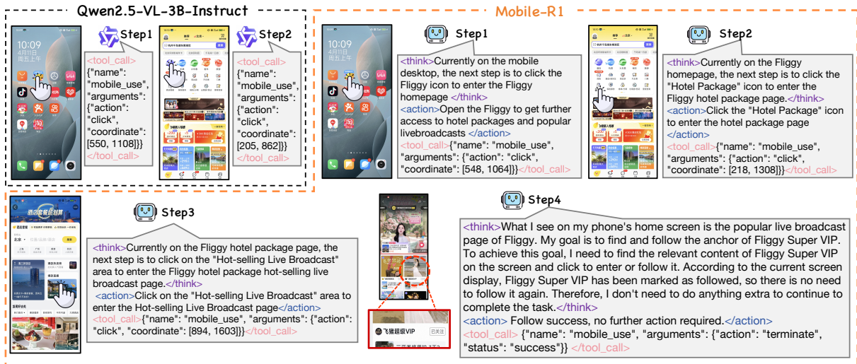
Figure 5: Comparison of reasoning trajectories between Mobile-R1 and Qwen2.5-VL-3B-Instruct on the task “Open Fliggy, enter the hotel package, enter the popular live broadcast, find Fliggy Super VIP, and follow the anchor”. In this case, Qwen2.5-VL-3B-Instruct failed at the second step, while Mobile-R1 completed the whole task accurately.
