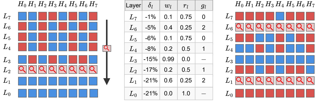
Figure 1: Illustrative application of BOSCH to a Transformer with L=8 layers and H=8 heads per layer, targeting \rho=0.5\% SWA heads. Left (Stage 1: layer-importance detection) : each row is a layer; blue squares are self-attention heads ( z=1 ), red squares are SWA heads ( z=0 ); light-red squares with a loupe indicate the layer(s) currently scored via black-box optimization, from top to bottom. Middle (Stage 2: adaptive ratio assignment) : for each layer \ell we compute the relative drop \delta_\ell (from the original model), normalize it to an importance weight w_\ell \in [0, 1] , and map it to a per-layer SWA ratio r_\ell while respecting the global budget. Right (Stage 3: multi-layer head selection under adaptive ratios) : layers are bucketed by ratio into groups g_\ell and optimized jointly from more SWA-tolerant to less tolerant; the example highlights searching layers with g_\ell=2 using r_\ell=0.25 , yielding the final head mask z . "—" indicates that either entire layer is full-attention or SWA (no optimization is applied).
