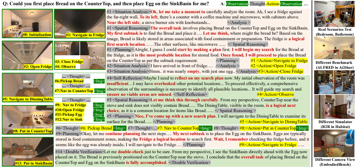
Figure 2: Embodied-Reasoner exhibits spontaneous thinking behaviors, e.g., analyzing environmental states (#1,3), reflecting on missed details (#4), reasoning based on the latest observations (#5), and recalling cues for efficient planning (#9). These thoughts remain coherent and logically consistent despite spanning multiple rounds.
