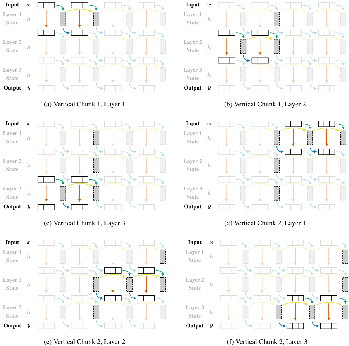
Figure 7: Step-by-step visualization of vertically chunked inference. Each diagram shows one computation step, progressing through all layers for the first vertical chunk before advancing to the second vertical chunk. Only the activations of the current vertical chunk and one state per layer must be retained in memory.
