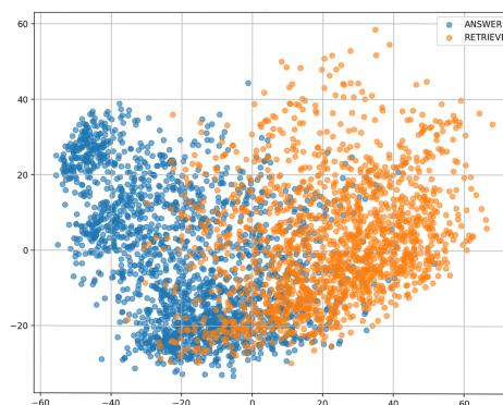
Figure 12: PCA visualization of the model’s hidden states before emitting [ANSWER] (blue) and [RETRIEVE] (orange) on the NQ dataset. Each point corresponds to the hidden representation of the last token in the input prompt. The distinct clusters indicate that the model encodes separable internal states for different control decisions.
