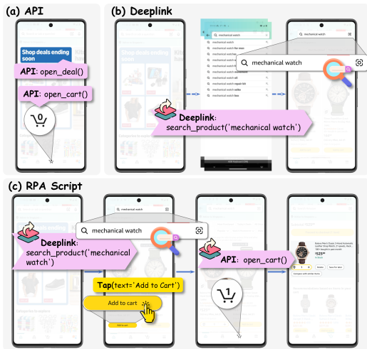
Figure 2: Functional Comparison of APIs, Deep Links, and RPA Scripts. The figure uses the Amazon app as an example: (a) the open_cart() API directly opens the shopping cart; (b) the search_product() deeplink directly performs a product search; and (c) an RPA script combines APIs, deep links, and GUI operations to automate a complete workflow.
