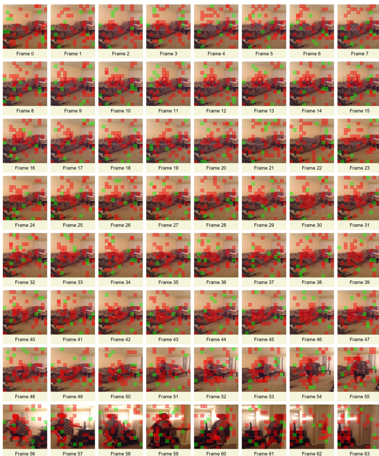
Figure 6: Visualization of the token selection strategy on a sample video clip. The red patches indicate high-relevance regions identified by the Semantic Scout, which aligns closely with the textual query regarding the person and the blanket. The green patches denote structural anchors retained by the Structure-Aware Compensation module to preserve global context. This hybrid approach effectively captures the core interaction while maintaining scene coherence.
