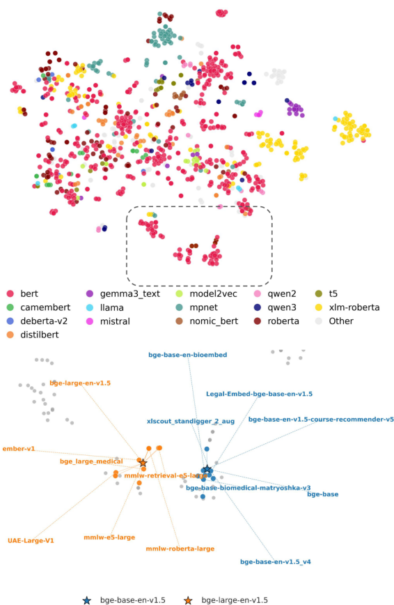
Figure 1: Map of Encoders. Top: Map for 1101 sentence encoders, visualised by t-SNE and coloured by the encoder type. Bottom: A 30% zoomed-in view of the dotted area showing the top-7 nearest neighbours for bge-base and bge-large . Nearest neighbours belong to the same primary architecture and are closely located.
