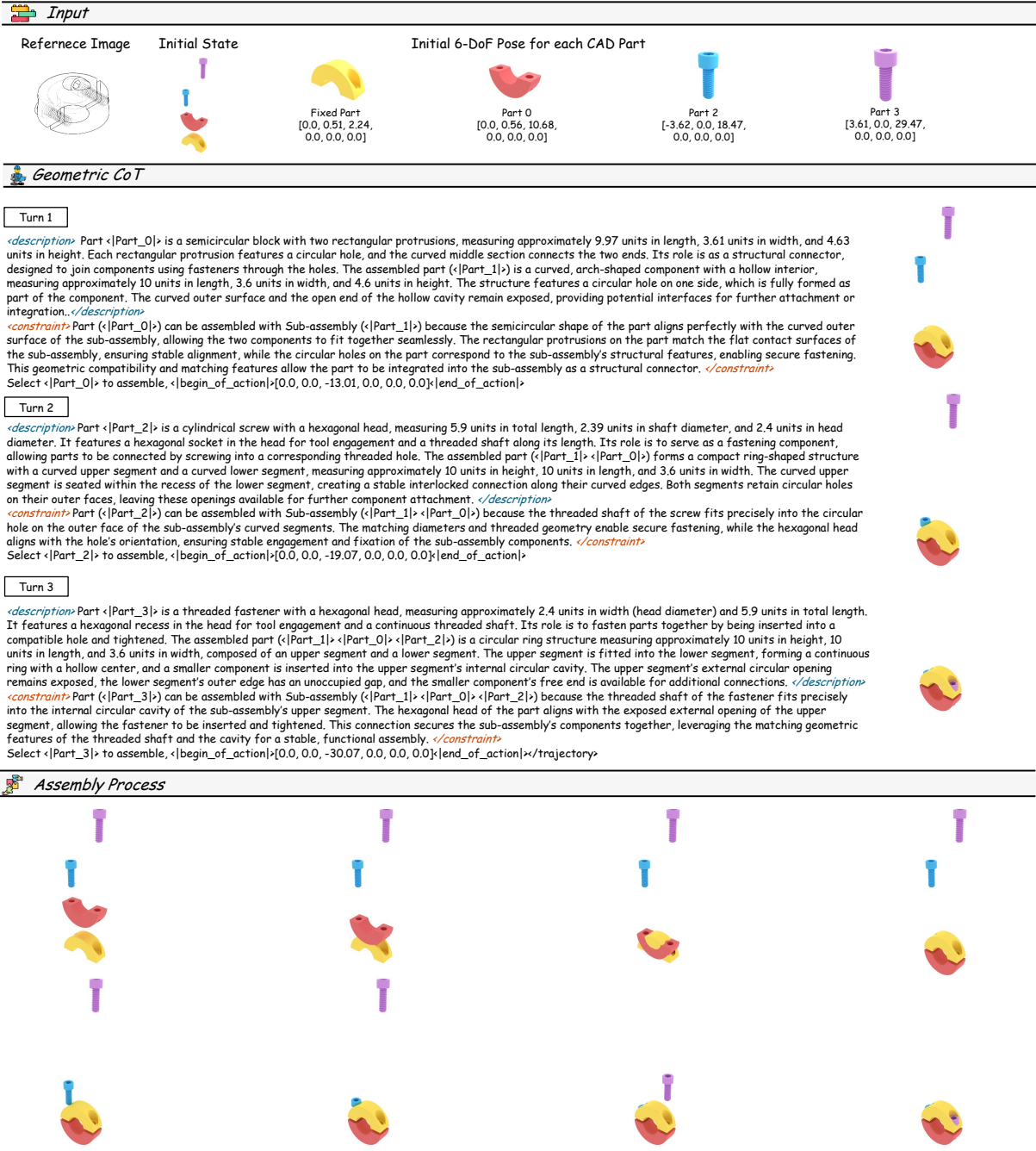
Figure 17: A representative failure case from CADMATE-8B. While the model correctly infers the assembly sequence, it produces physically implausible motions with inter-part penetrations during intermediate steps. It illustrates that physical collision avoidance remains a significant challenge for current MLLMs.
