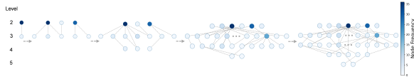
Figure 16: The tool graph evolution diagram of DA-Bench. In this diagram, each node represents a tool function, and the edges represent the invocation relationships between tools. The darker the color, the more frequently the tool is invoked.
