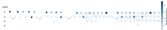
Figure 18: The tool graph evolution diagram of MATH. In this diagram, each node represents a tool function, and the edges represent the invocation relationships between tools. The darker the color, the more frequently the tool is invoked.
