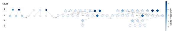
Figure 19: The tool graph evolution diagram of TabMWP. In this diagram, each node represents a tool function, and the edges represent the invocation relationships between tools. The darker the color, the more frequently the tool is invoked.
