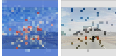
Figure 8: Question-conditioned pruning visualization. For the same image, MVP-Token retains different visual tokens according to different questions. For the heatmaps, red indicates high importance, while blue indicates low importance.
