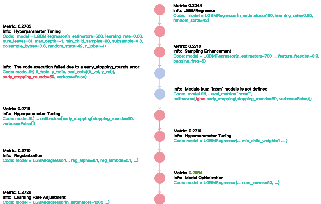
Figure 6: Detailed OPT-Agent-ML Trace on the Bike Sharing Demand Task , utilizing gemini-2.0-flash as LLM base model. The red, and blue nodes represent the improve, and debug action, respectively.
