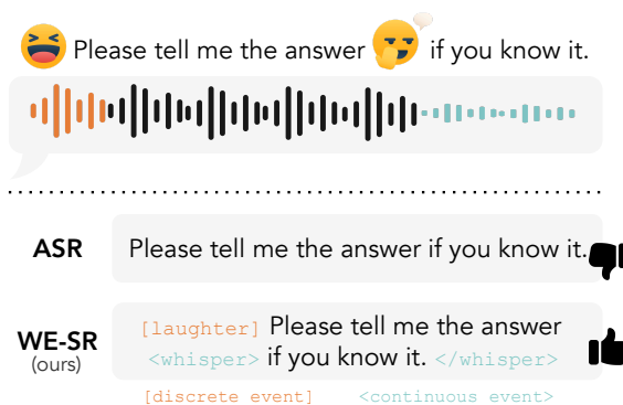
Figure 1: Task overview of our WESR that generates transcripts with explicit word-aligned continuous/discrete event tags.
