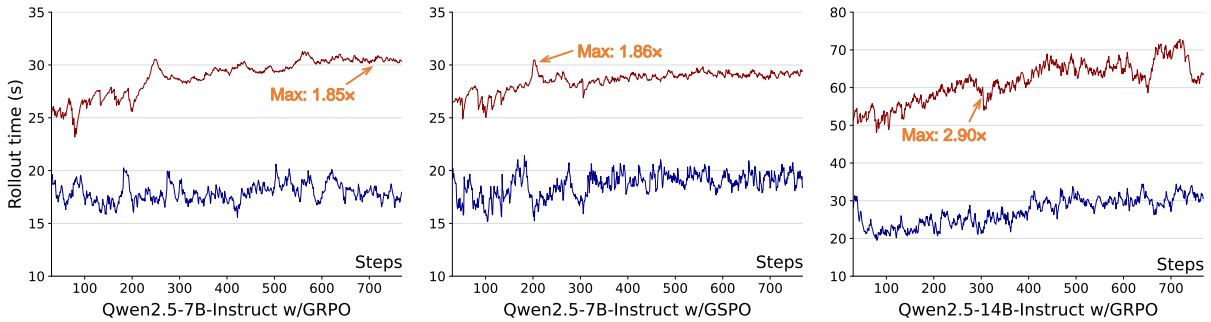
Figure 4: Comparison of rollout time across different models and algorithms in the math task. The upper curve shows the per-step rollout time without MTPs, while the lower curve shows the per-step rollout time under MTP-RL.
