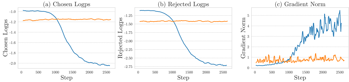
Figure 6: Training dynamics of SimPO on High Average and Low Average subsets—(a) log-probabilities of chosen responses, (b) log-probabilities of rejected responses, and (c) gradient norm over training steps. The colored lines represent data selection strategies: High Average (blue), Low Average (orange).
