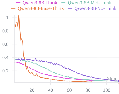
Figure 6: Entropy during GRPO. We compare Qwen3-8B-Base trained in the Think mode with Qwen3-8B trained under Think, No-think, and Mid-Think modes. The panel plots entropy versus training steps. Notably, Mid-Think both increases training entropy.
