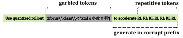
Figure 6: A mid response error propagates to future tokens. Although the initial garbled tokens are clipped, the repetitive tokens induced by this error are not clipped by token-level objectives.
