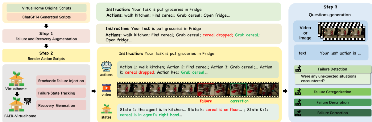
Figure 3: Data generation workflow: (1) rule-based augmentation of VirtualHome scripts with 3 failure events (Drop, Grab-Failure, Find-Failure) and recovery actions; (2) multimodal rendering via FAER-VirtualHome, generating synchronized first/third-person videos, action sequences, and state snapshots; (3) creation of 12k Q&A pairs for four failure-reasoning tasks, with a test set balanced across failure/normal cases and unseen scenes.
