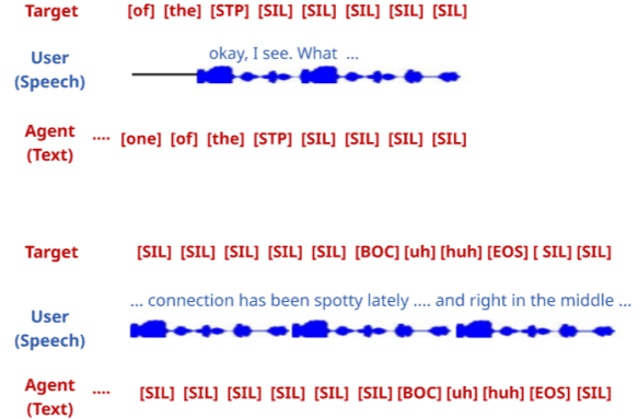
Figure 3: Training examples for duplex control tokens. Top: the agent emits [STP] when interrupted by the user. Bottom: the agent emits [BOC] to produce a backchannel during user speech.
