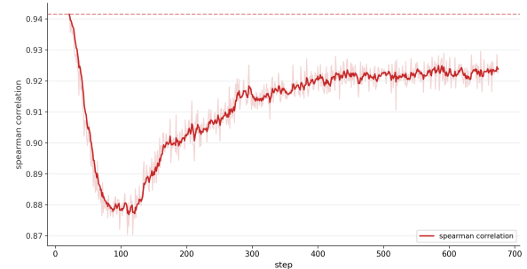
Figure 6: Off-policy diagnostic. Spearman rank correlation between \pi_\theta -based and \pi_{\text{old}} -based suffix-entropy scores, averaged across prompts during training.
