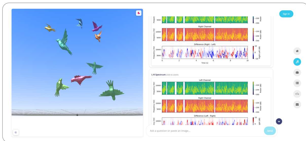
(b) This display shows the L-R spectrum, with the bottom graph highlighting frequency differences and channel bias between left and right. The bird icons appear slightly enlarged due to the collapsed GUI sliders at the bottom-left. Flight trails, trail points, and axes are hidden, and the view is zoomed in and angled slightly upward.
