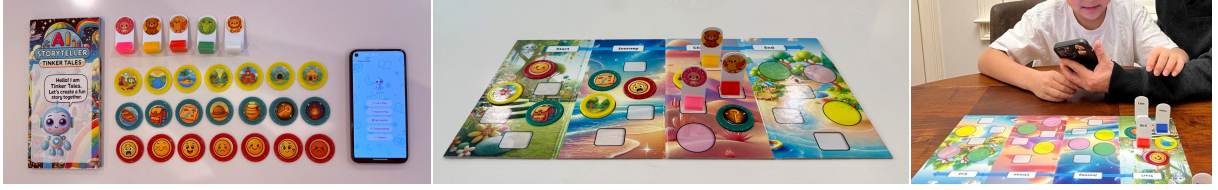
Figure 1: Overview of Tinker Tales . Children iteratively develop and refine stories through interaction with a conversational AI while placing and moving tangible story elements on a physical board. A mobile app mediates this interaction by sensing NFC-embedded story elements and supporting voice-based dialogue.
