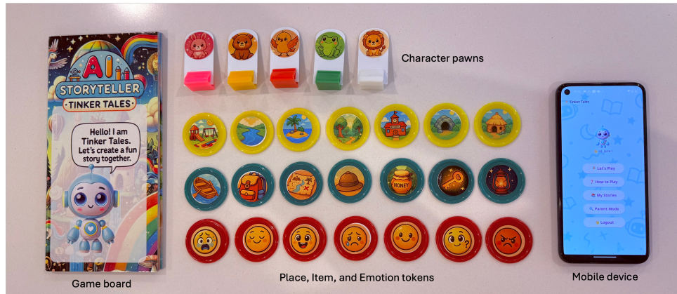
Figure 8: Physical setup of Tinker Tales . The system includes a storytelling board structured into four narrative stages, NFC-embedded character pawns and place, item, emotion tokens, and a mobile device that mediates voice interaction and NFC-based input. Each pawn and token is labeled on the reverse side with a corresponding word representing the story element.
