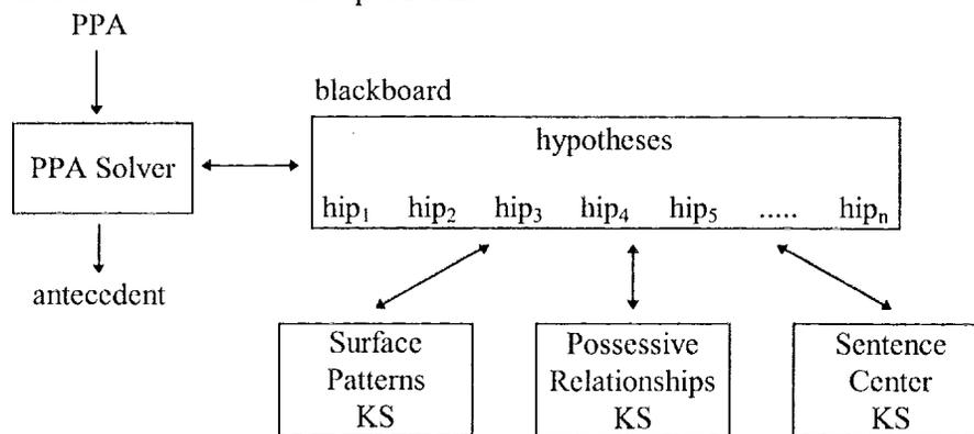
Figure 1 - a distributed architecture for PPA resolution
