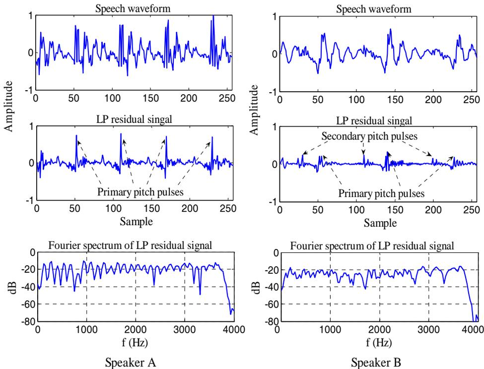
**Figure 1.** Examples of speech waveforms and LP residual signals of two male speakers. Left: Speaker A; Right: Speaker B; Top to bottom: speech waveforms, LP residual signals and Fourier spectra of LP residual signals
