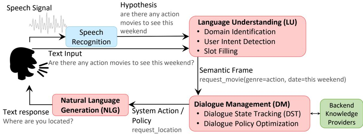
Figure 1: Pipeline framework of spoken dialog system.
