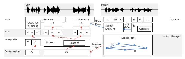
Figure 3: Incremental Units at different levels of processing. Some grounded-in relations are shown with dotted lines. W=Word, SS=SpeechSegment, SU=SpeechUnit, CA=Communicative Act.
