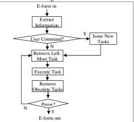
Figure 2. The Main Loop of the DM.
