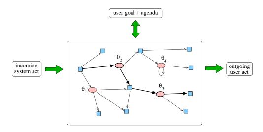
Figure 1: User simulator viewed as a 'decision network': square nodes indicate deterministic decision points; round nodes indicate random decision points, and have associated parameters  $\theta_i$ ; the loop on one of the nodes indicates it has a geometric distribution associated with it.
