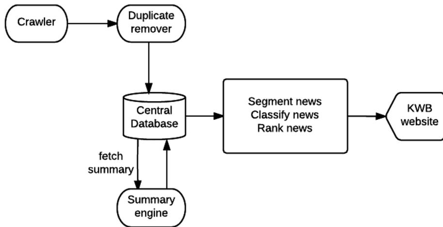
Figure 1: The architecture of KWB
