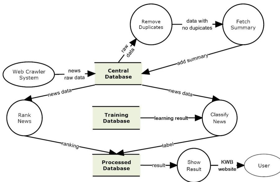
Figure 2: The data flow diagram of KWB
