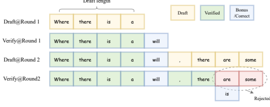
Figure 3: A mini-sample of QSPEC, where yellow, red, and blue tokens represent W4A4 draft tokens, rejected tokens, and tokens generated directly by W4A16, respectively. While these green ones are draft tokens that have been verified and accepted by W4A16.
